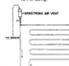
Fig. 2-4. Installation of automatic air vent on panel coil.
